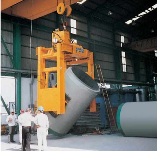
Gantry Crane Rotating Clamp for Pipes PWG-R
