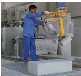
Swivelling suction plate with pneumatic cylinder ESP-SW-P
