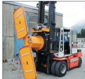
Vacuum Turning Device for Fork Lift Trucks
