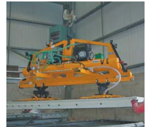
Vacuum Spreader Bar VT-6000-D for crane operation
