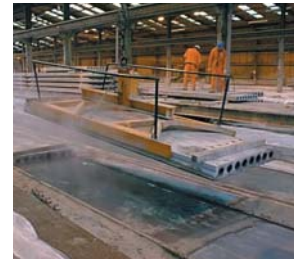
Laying Clamp for Hollow Core Slabs VZ-D
