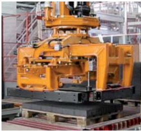
Electric Cubing Clamp ATZ-E-4
