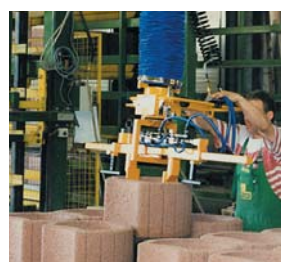
Vacuum Hose Lifter with Pneumatic Clamp ASZ-P
