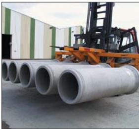
Hydraulically Adjustable Multiple Forks MFD-UNI
