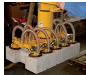
Multiple suction plate for gutter blocks
