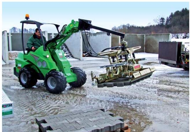
Installation clamp in combination with Mini-excavator
