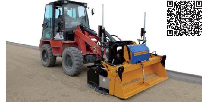
As against conventional screeding blades the LEVELKING work with integrated smoothing board. With this function it is possible to screed not only the subbase, rather the top bedding for paver laying. The LEVELKING screed fully automatic controlled, accurate, fast and efficient – with no multiple transits. This makes the LEVELKING LK an efficient and affordable alternative.
