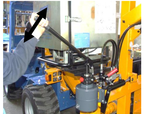
Actuating the hand pump lowers the mast.
