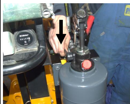
Move the adjusting lever on the hand pump to position I
