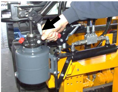
Move the red setting lever to position A
