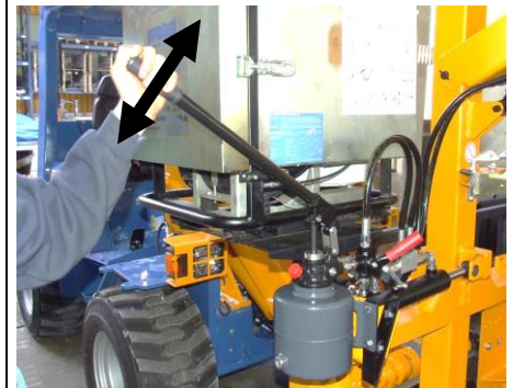
Actuating the hand pump raises the mast.
