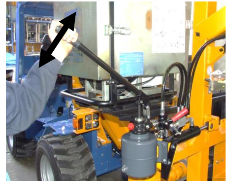
Actuating the hand pump lowers the mast.
