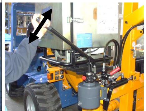
Actuating the hand pump moves the mast to the left.
