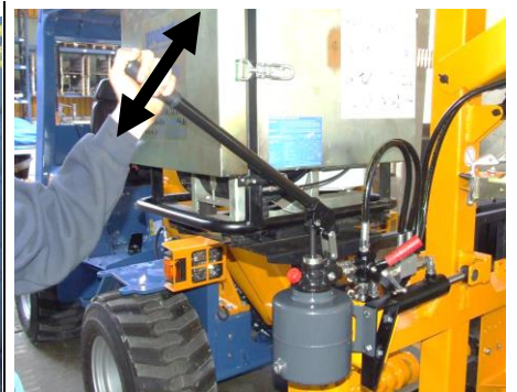
Actuating the hand pump moves the mast to the right.
