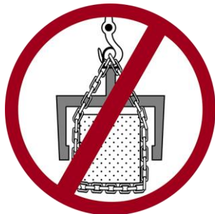
Load securing chain (lashing chain) must not be used as sling chain! The load securing chain can break and the load would fall! Risk of injury and death!
