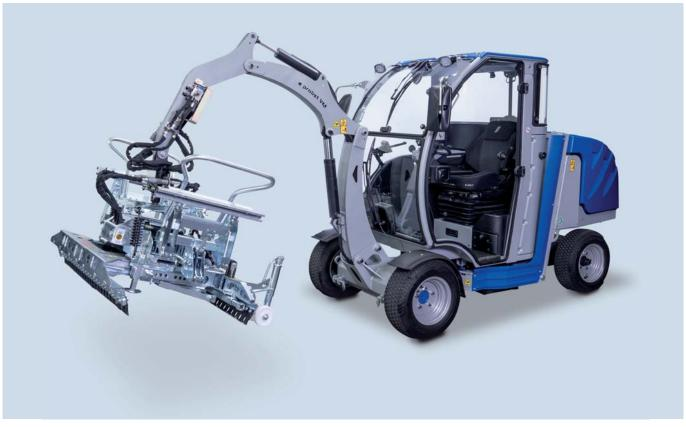
VM-X-PAVERMAX premium with HVZ-UNI-II (picture with accessories LED light package and exterior mirrors)
