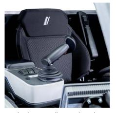
Joystick with ergonomically arranged controls
