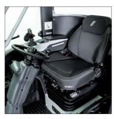
Decoupled driver's cabin with air-suspended comfort seat, seat heating and longitudinal damping
